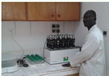
*Automatic Methane Potential Test System to assess the biochemical methane potential of bio-wastes, located at the ISRA/IRD research centre of Dakar, Senegal (September 2015). © J.-M. Médoc*
