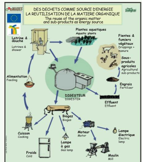
Poster explaining the re-use of bio-waste (i.e. organic matter) as inputs in a biogas plant to produce energy and fertiliser.
